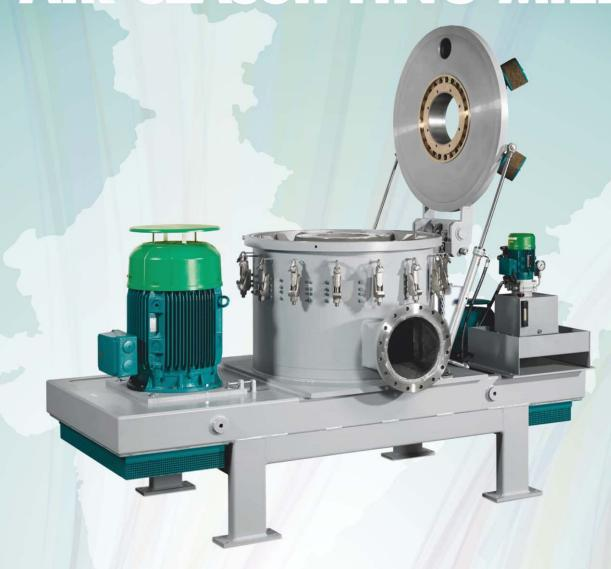
The YAGNM Air classifier Mill (ACM) is an air classifying mill with integrated grinding, classifying, conveying, and collecting functions for achieving ultra-fine grinding (up to 2 micron\*) based on the type of product
